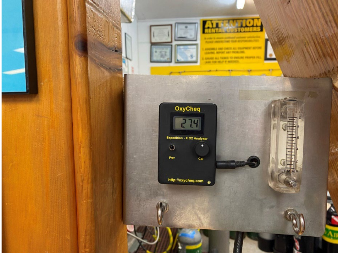
Figure 5: Inspection of Oxygen levels in Passenger 1's diving tank. (October 9, 2023/USCG)
